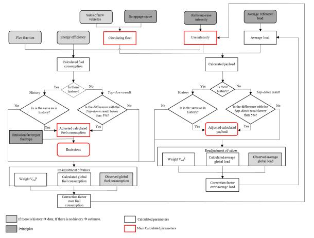
Figure 4. Procedure adopted to estimate energy consumption using the *bottom-up* methodology. Source: Made by the authors.
