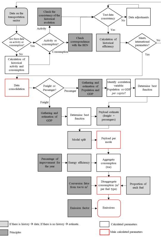
Figure 3. Procedure adopted to estimate energy consumption using the top-down methodology.
